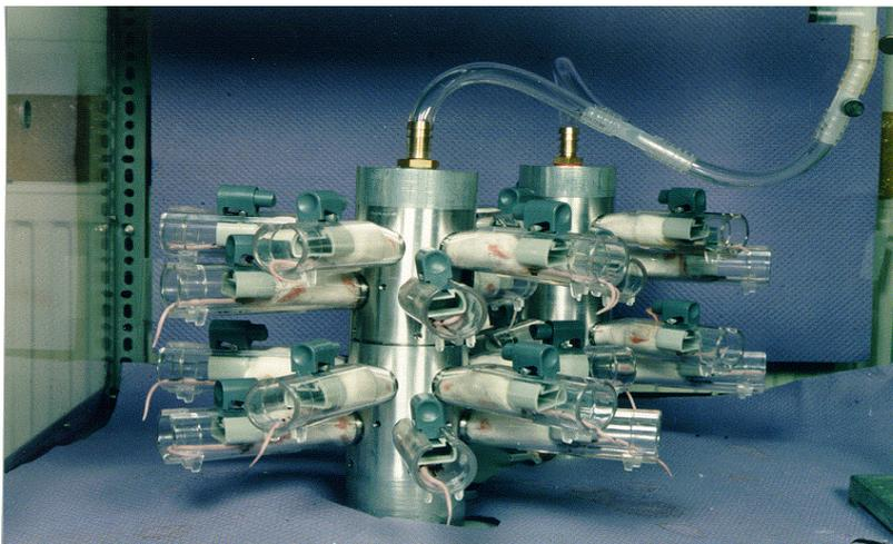
Figure 1 Experimental set-up for nose-only exposure. Mice are restraint in a tube (A) and are attached to the exposure chamber (B). Vehicle or fragrance were either vaporized by maximum vapour pressure or nebulized in acetone to produce an aerosol of liquid droplets
