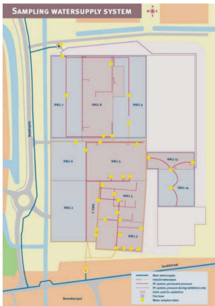
Figure 1: The layout of the auction building where the West-Frisian Flora was held, indicating the watersupply system and all sampling points of the watersupply in the environmental investigation.
