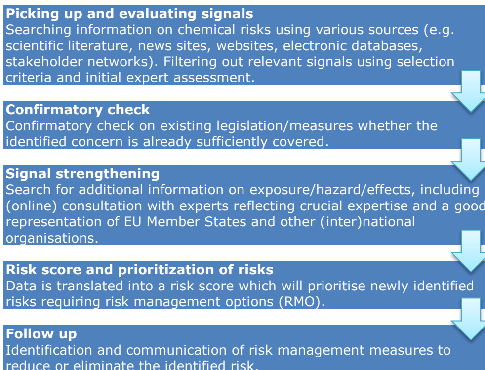
Figure 1. Components and steps involved in an early warning system as developed for New or Emerging Risks of Chemicals (NERCs) [5].
